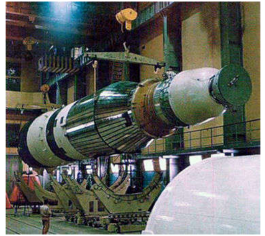
Zond mounted on top stage of Proton booster in assembly hangar
